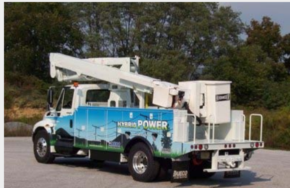
Odyne Plug-In Hybrid Aerial Lift Truck (8-hour zero-emission operation)
